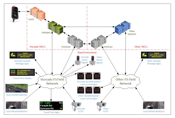
Figure 4.2 Current generic system-to-system architecture
