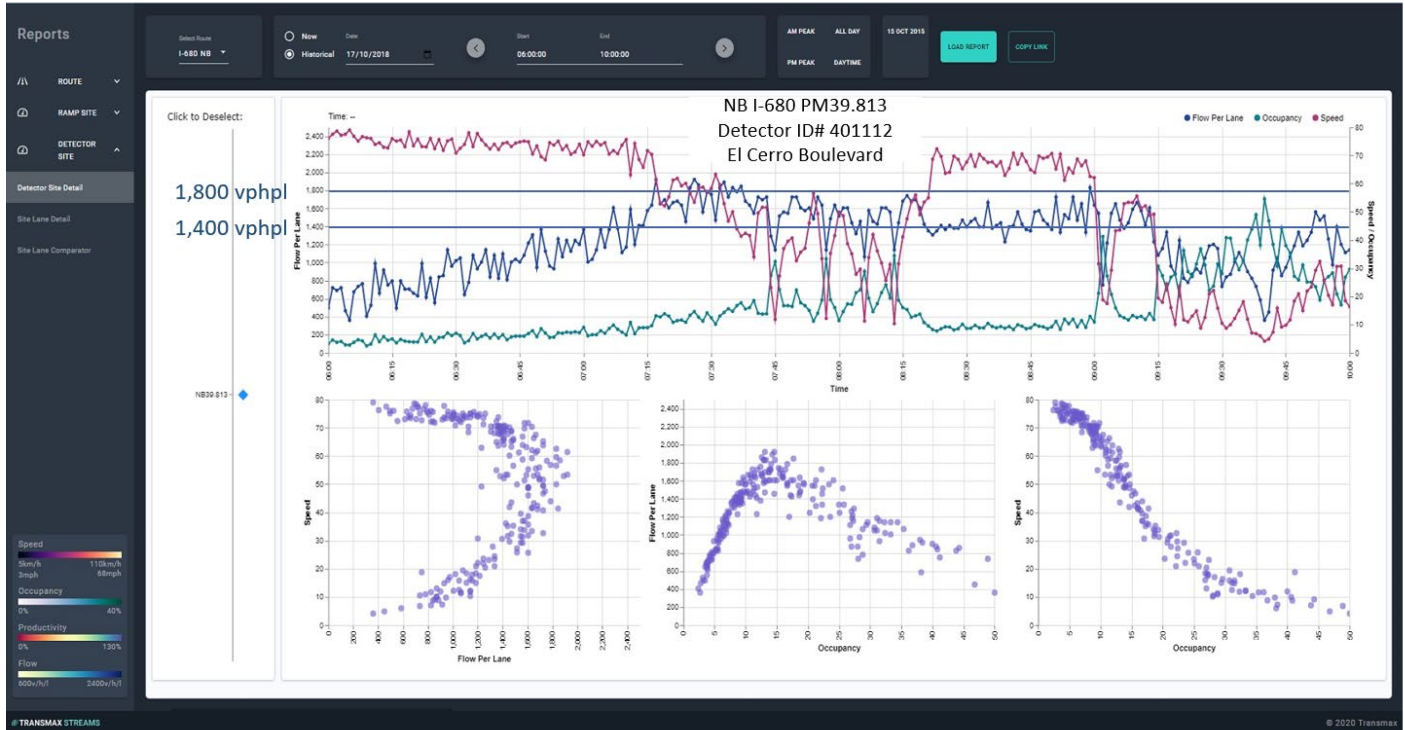
Figure 4-4 I-680 Northbound at El Cerro Blvd – Traffic Flow Characteristics
